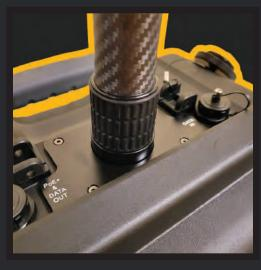
8. Connect the remaining poles. Unscrew the cap at the top of the case and screw in the lower pole assembly.
