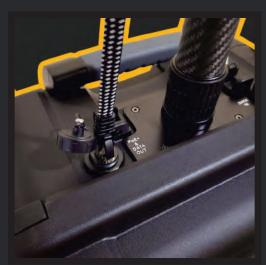
10. Connect the other end of your ethernet cable to the ethernet port labeled "PoE+ & data out"
