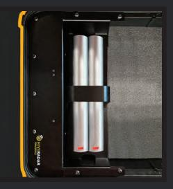
2. Insert the Ventev - Ven-Volt 2 batteries into the battery chasis.
