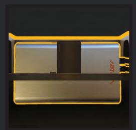
3. Plug in the POE OUT cable to the PoE Output port, if planning to connect the AP to data backhaul, plug in the DATA IN cable to its LAN port.
