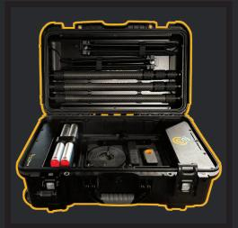
**4.** Remove the stabilizer legs, poles, mounng bracket, ethernet cable and any other tools you'll require for your survey.
